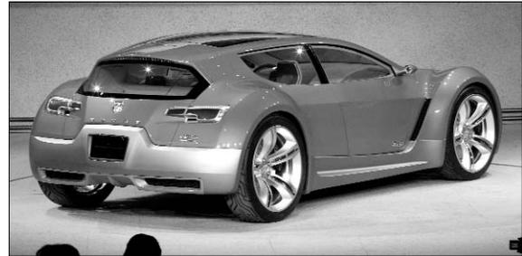
The Dodge ZEO Concept (above) is an all-electric “2+2” sport wagon with rear wheel drive, what looks like the same 200 kW motor as the other two, but a 64 kWh li-ion battery that gives 250 mile range. With a curb weight of 3400 lbs it hits 60 in 5.7 s, does the quarter in 11 s even, and hits 130 mph.
