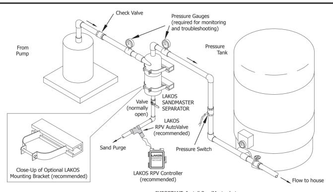
IMPORTANT: Install SandMaster between the check valve and pressure tank.
