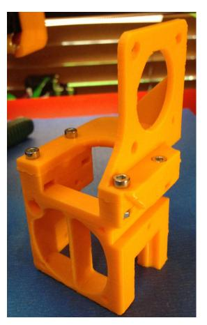
Make sure you have the (3) Titan Extruder to motor through holes to the motor temporarily so extruder position will be true. These just need to be loose and pushed through the base mount for positioning.
