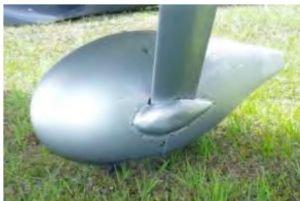
New Demo has a "clean" wheel pant installation.
