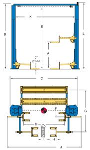
Rise is measured with adapter in highest position.
