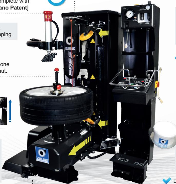
Two **LASER POINTERS** allow to easily set working tools in proper position simultaneously, according to tyre diameter and width. Once the rim position is set, you never have to change anything in your operation.
