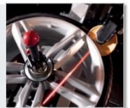
Bead breakers tower moves in synch with clamping chuck, thus guaranteeing best bead breaker angle on disks, with any kind of tyre.
