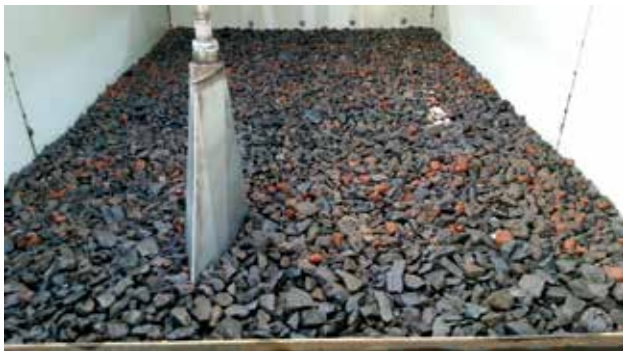
The photo at left shows the successful stratification of a difficult material with a Snoby Separation Systems wet jig. At right, the red pumice is jigged to the top of the bed.
