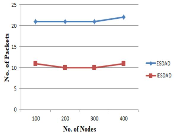
Fig. 5 Packet loss comparison
