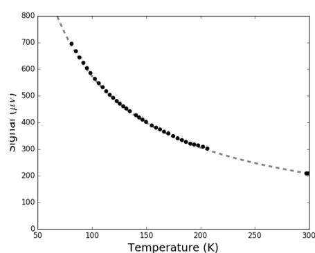
Fig. 5: A relative measure of the susceptibility signal from a gadolinium-oxide [ $\text{Gd}_2\text{O}_3$ ] sample, as a function of absolute temperature  $T$ . The vertical scale gives the rms measure of the a.c. signal at the lock-in's input.
