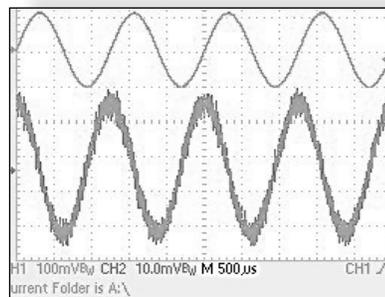
Fig. 3: (Upper trace) A monitor-voltage waveform proportional to the current  $i(t)$  in the primary coil; (lower trace) The net emf from the anti-series-connected secondary coils, when a ferrite-bead sample is centered inside one of the secondaries.
