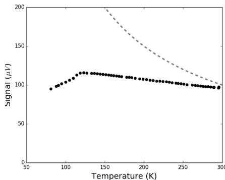
Fig. 6: Susceptibility signal vs. absolute temperature for a manganese-monoxide [ $\text{MnO}$ ] sample. The dashed curve shows a  $1/T$ -dependence that does *not* fit the data, either above or below 120 K.
