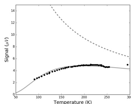
Fig. 7: Susceptibility signal vs. absolute temperature from a copper-acetate [ $\text{Cu}_2(\text{CH}_3\text{COO})_4 \cdot 2\text{H}_2\text{O}$ ] sample. The solid curve shows the results of a copper-dimer model of two interacting spin-1/2 atoms.
