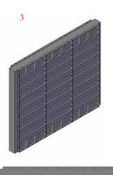
Slide the CIP Window onto the wall ties in the desired location.
