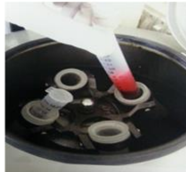
FIG 2: PLACING THE BLOOD IN THE CENTRIFUGE AND CENTRIFUGING AT 3000RPM FOR 10 MINUTES
