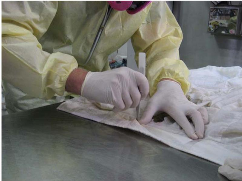
9. Bulk samples were cut from sewage-soaked padded items, including this quilted winter vest, before cleaning. Both layers (fabric and padding) were removed for sampling.
