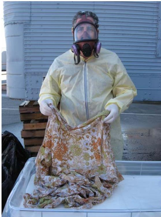
7. A number of uncontaminated contents were sampled prior to and after cleaning in order to determine if cleaning sewage-impacted items cross-contaminated other laundry items. No cross-contamination was observed when the extra heavy wash cycle was used.
