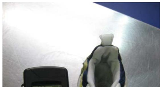
13. 100 cm.<sup>2</sup> samples were collected from two sides of the same shoe for pre- and post-sampling. The work boot showed a low level of residual contamination after cleaning.
