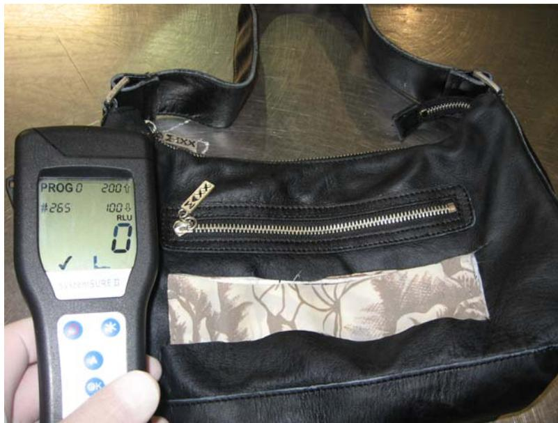
11. A sewage-soaked leather purse was sampled with a portable ATP field test system. Note the 100 cm.<sup>2</sup> patch that was cut out for laboratory sampling.
