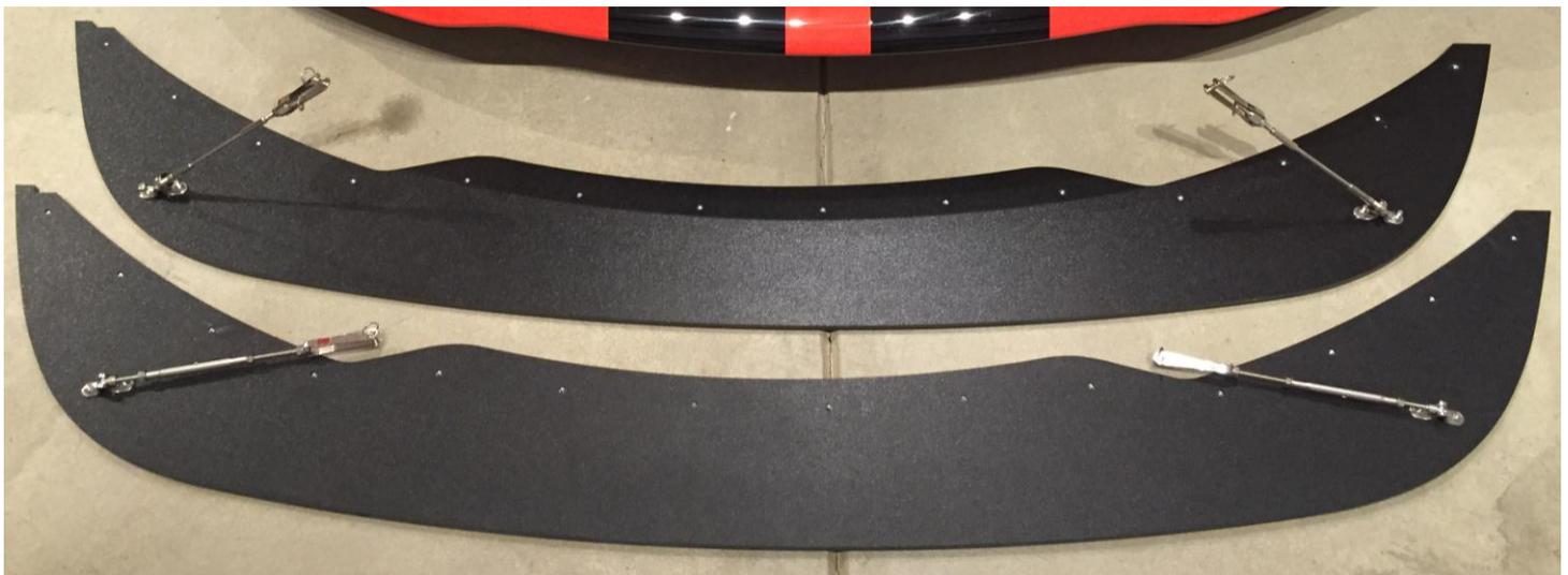
**DSE ACR-E Splitter Extension and Strut Assembly (bottom) vs. OEM (top)**
