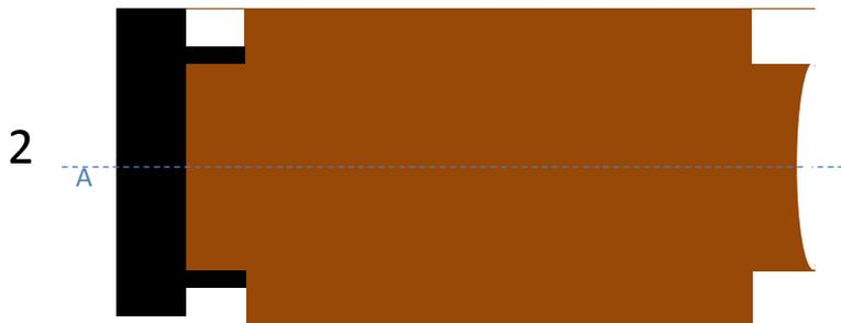
Cut the top of the candle holder shelf, where the metal holder will attach. (known as the Bobèche, for catching wax). Cut the diameter to the size of the cap that will fit over it so it fits very snug. Sand the top smooth. Mark the center now with a small dimple for a drill later.
