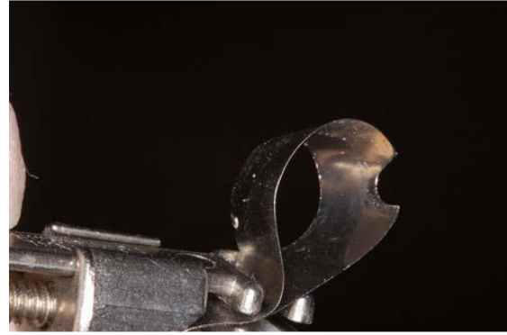
Fig10: Contact cut away with a small football finishing carbide.
