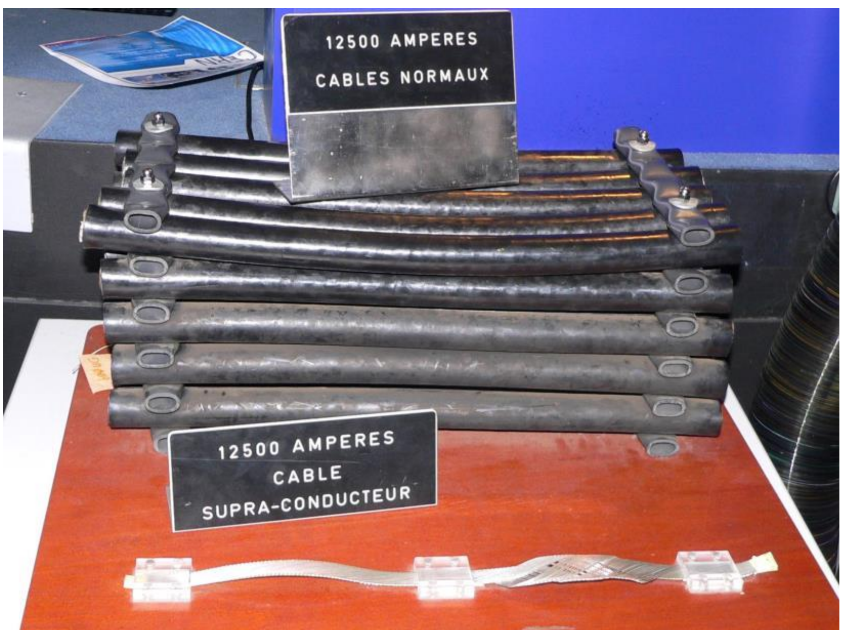
Cables with the same current rating: 12,500A
