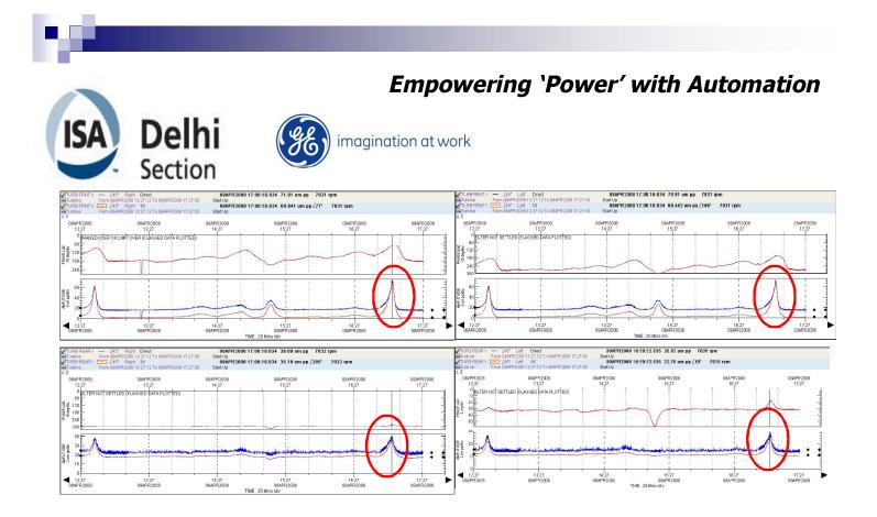
Rise in direct/1X amplitudes can be seen with different amplitude levels on both Turbine Front & Rear Bearings
