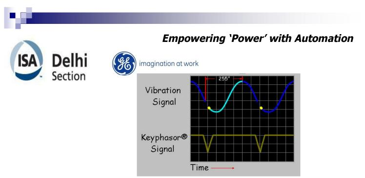
Absolute phase angle is measured for filtered, integer multiple frequencies of running speed. Such as 1X, 2X etc..
