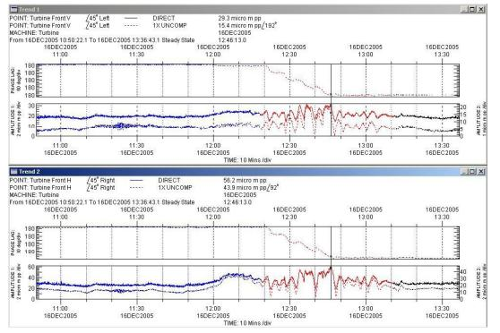
Fluctuations in direct/1X amplitudes with significant change in 1X phase can be seen here
