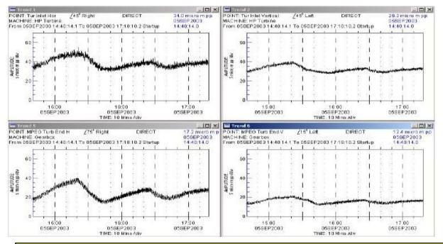
Cyclic vibrations were on account of varying 1X vibrations
