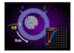
From 0 degree reference, Absolute phase angle is measured at a point on rotor, which is closest to reference transducer or say is showing maximum positive peak in vibration signal. This is lagging phase angle and is identified in the direction opposite to direction of rotation.
