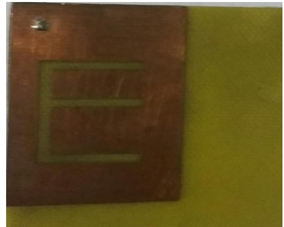
Fig.12: Fabricated antenna Top view
