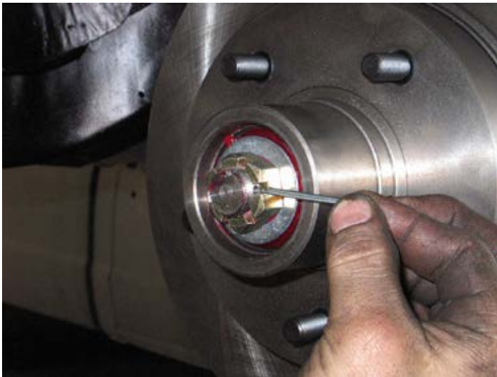
The discs are slid onto the spud of each spindle.
