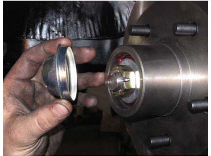
Finally, dust covers seal off the brake discs.
