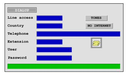
Once the phone number has been entered, it is possible to make a call by selecting the telephone icon and pressing [ENTER] or by pressing the "CALL" softkey. Likewise, to hang up, it may be done using the icon or the "hang up" softkey.
