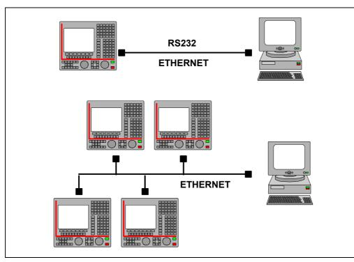
For the RS232 connection, the remote PC must have the WinDNC software (version V2.00 or later) installed in it. For the Ethernet connection, the remote PC must have the WinDNC software (version V4.00 or later) installed in it.
