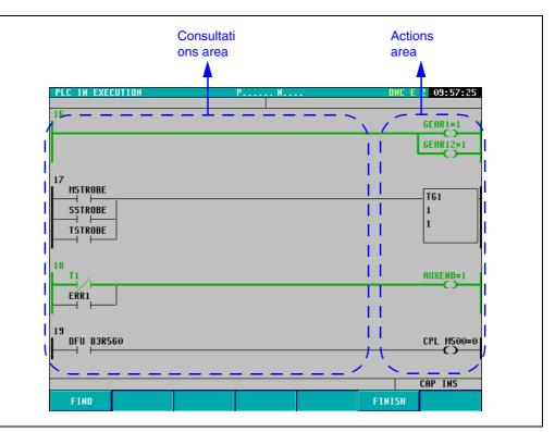
As shown in the figure, the instructions of the PLC program in ladder language is made up of elements connected to each other by segments. It also shows the logic way for the flow highlighted with a thicker green line and shows the values of registers, timers, counters, etc.
