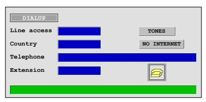
Once the phone number has been entered, it is possible to make a call by selecting the telephone icon and pressing [ENTER] or by pressing the "CALL" softkey. Likewise, to hang up, it may be done using the icon or the "hang up" softkey.
