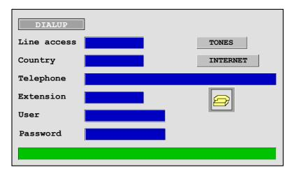
Once the connection has been made, the bottom of the screen will show the IP address. This address must be communicated to the person who is going to telediagnose from the PC.
