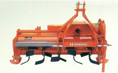
Offset can be achieved by turning a simple handscrew. All sliding members are galvanised to avoid corrosion and ensure a smooth sliding action.
