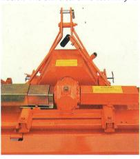
Top mast and 3 point linkage is independent from the gearbox, eliminating all shock loads on the drive assembly.
