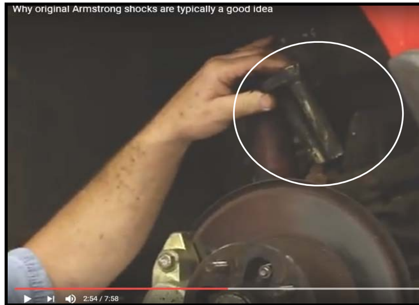
Figure 36 - Damaged Support Bracket
