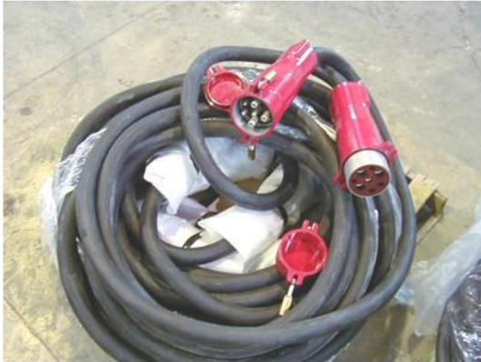
240 Amp x 1 kV Power Cords
