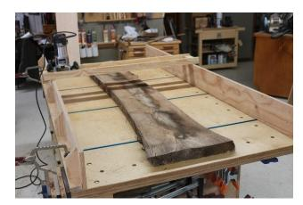
The jig is constructed from ¾" plywood
