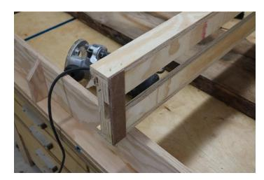
Include a stop on the bottom of the gantry to prevent the gantry from sliding off the rails
