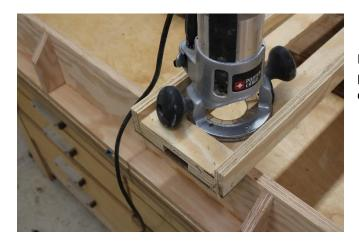
Include a stop at both ends of the gantry to prevent the router from falling off, or the bit contacting the rails.
