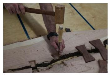
Use a chisel to remove the waste, cutting to the layout line. Test the fit frequently. The bowtie should easily tap into the recess.
