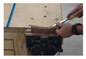
Use a hand chisel to pare down to the layout line. Work downhill on all the cuts, toward the waist of the bowtie. Be careful to not angle the edges.
