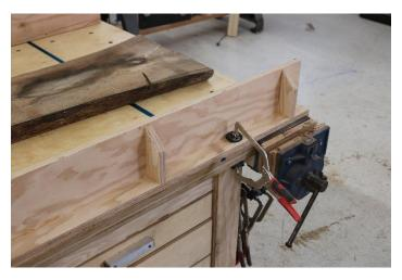
Gussets glued and fastened between the horizontal and vertical surfaces keep the parts square, and add rigidity.
