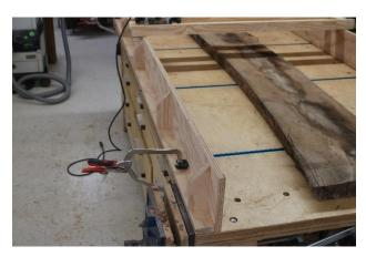
Clamp the rails to a workbench or sheetstock. The rails are 6" tall. Make the length to suit your needs.
