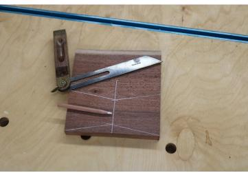
A 12-degree angle works great for the bowtie/dovetail. Use a charcoal pencil for good visibility on dark wood.
