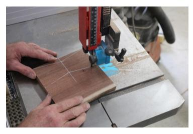
Use a bandsaw, jig saw or handsaw to cut the shape. Stay outside the lines.
