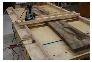
Lay the rails in the other direction for thinner slabs.
