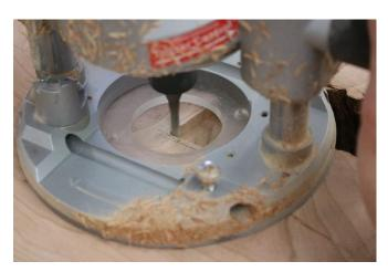
Use a plunge router freehand to excavate the bowtie socket. A ¼" upcut spiral works well. Set the depth slightly less than the thickness of the bowtie. Get as close as you can to the layout lines, but don't go outside them.
