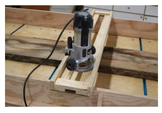
Make the gantry to fit your router. If you're using a large diameter bit, you'll need a variable speed router.
