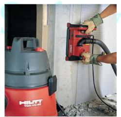
tool, capturing hood, tubing. Use an extraction specification (ie H (High) M Class filter unit). Don't just commercial vacuum.
