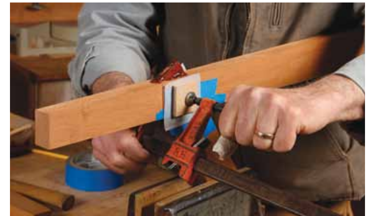
Glue and clamp. This is an outdoor chair, so Hare uses epoxy for his glue-up. Because the leg joint is so visible, he tints the epoxy there with mahogany sanding dust to more closely match the chair. He sizes the joint with a straight epoxy mixture and then adds the dust and applies the tinted epoxy. The mahogany dust, like the microfiber, adds strength.
