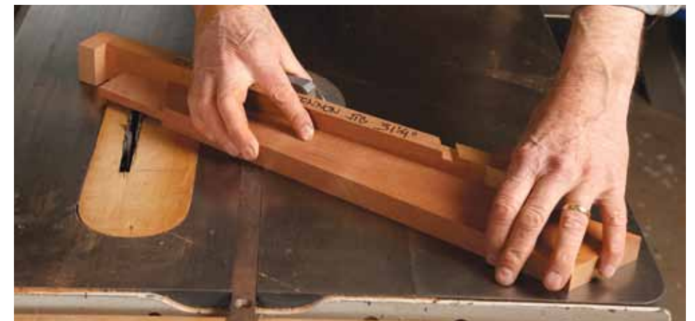
Glue and clamp. This is an outdoor chair, so Hare uses epoxy for his glue-up. Because the leg joint is so visible, he tints the epoxy there with mahogany sanding dust to more closely match the chair. He sizes the joint with a straight epoxy mixture and then adds the dust and applies the tinted epoxy. The mahogany dust, like the microfiber, adds strength.
