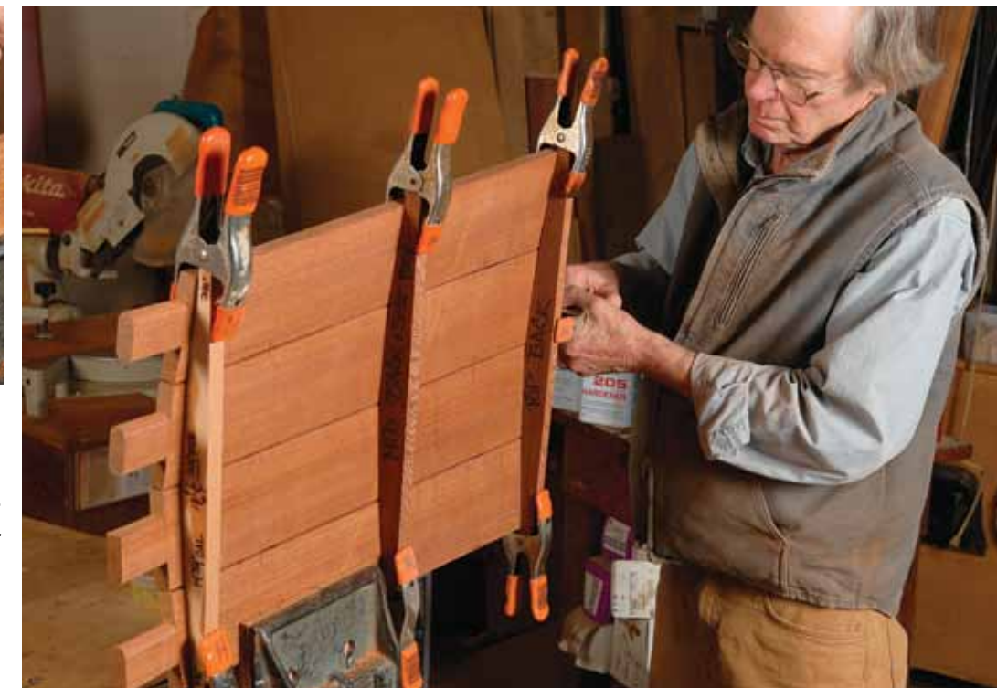
Separate slat assemblies for the seat and back. Using biscuits and epoxy with a microfiber additive to increase structural integrity, Hare glues up the back slats. He clamps the assembly using curved cauls so the back has a curved shape when the epoxy dries. He'll do the same with the seat slats.
