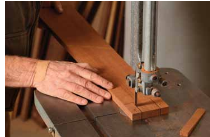
Cut the tenons. Hare cuts the tenons on the bandsaw, but they can easily be cut by hand. Once they're cut, use a rasp and file to round them.
