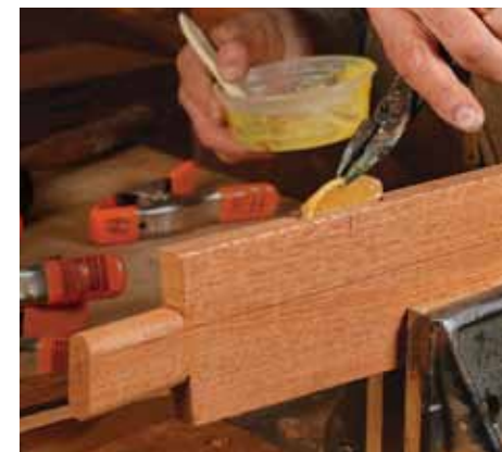
Separate slat assemblies for the seat and back. Using biscuits and epoxy with a microfiber additive to increase structural integrity, Hare glues up the back slats. He clamps the assembly using curved cauls so the back has a curved shape when the epoxy dries. He'll do the same with the seat slats.
