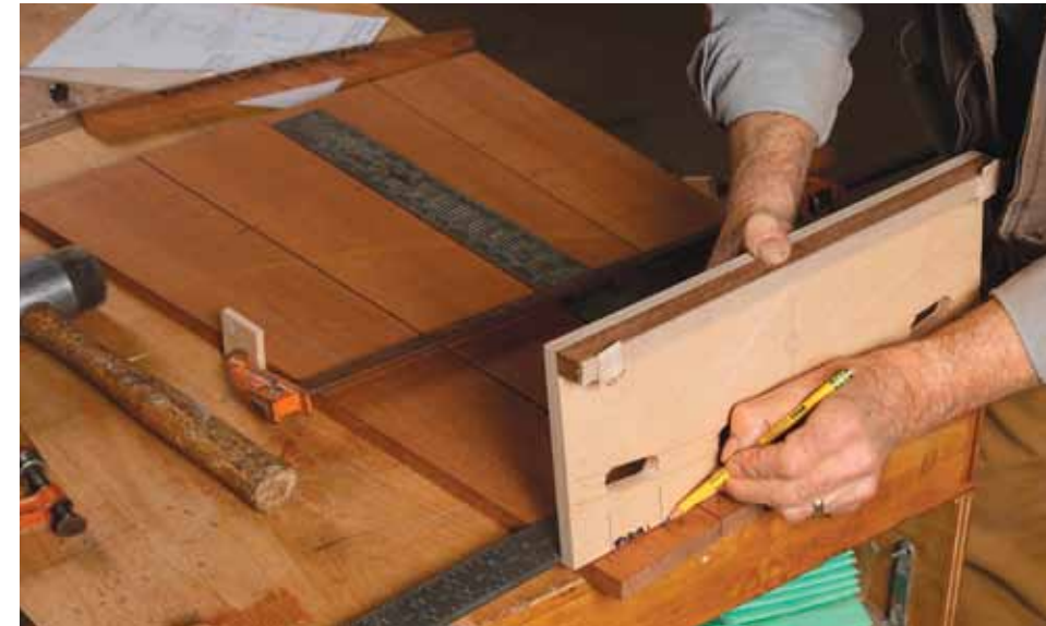
Mortising jig helps lay out tenons. While the back slats are dry-fitted and clamped, use the mortising jig from the seat slats to transfer layout lines for the tenons onto the back slats.
