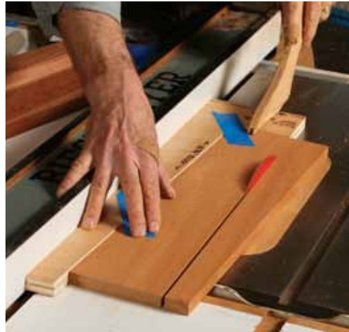
Start with a single-sided taper. An angled plywood jig holds the workpiece in place as Hare rips the taper on one side of each slat.
