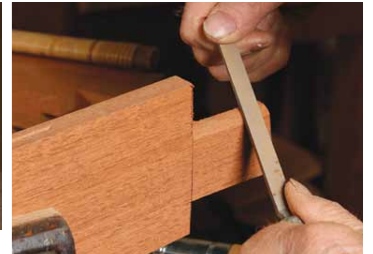
Cut the tenons. Hare cuts the tenons on the bandsaw, but they can easily be cut by hand. Once they're cut, use a rasp and file to round them.
