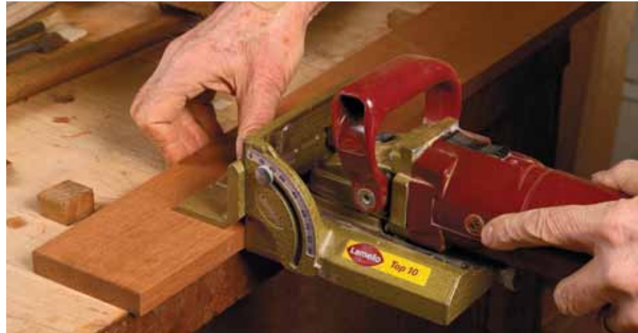
Biscuits do triple duty. The biscuits locate the seat and back slats front to back. They also lock all four slats into one assembly. Finally, by cutting a #10 slot and using a #20 biscuit, they create a consistent gap between the slats. Adjust the #10 setting so the resulting gap is \frac{1}{16} in.
