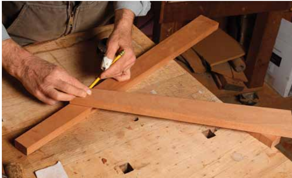
Marking mortise location. Once the legs are tapered with the same type of jig used to taper the seat and back slats, mark the location of the mortise on the front leg. Position the back leg on the front and pencil its location onto the front leg.
