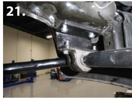
**15.** Install new front sway bar drop brackets using the provided  $3/8" \times 1"$  bolts. Install the factory sway bar mounts onto the new drop brackets using the factory hardware. (pic 20-21)
