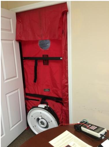
**Building Enclosure Testing is a value-added diagnostic procedure that identifies how much a building leaks air. The higher the rate of leakage correlates directly to higher energy costs.**
