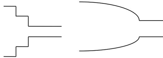
Fig. 2: Step taper. Fig. 3: exponential tapers
