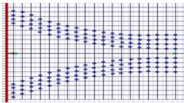
Fig. 7: Photonic crystal concave Taper
