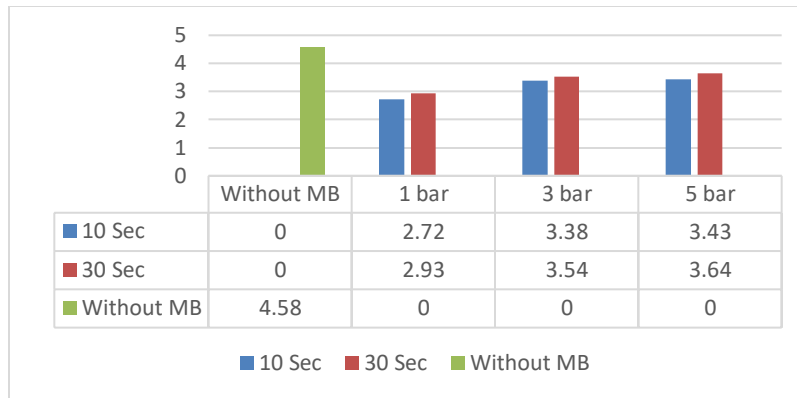
Fig. 9. Graph of the co-efficient of wear of Ti-N coating with time of exposure.
