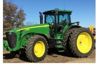
2007 John Deere 8330 MFD 4788 hrs, rear duals 480 80R50, front 420/85R34, Hydraulic 60 gpm pump, 4 outlets
