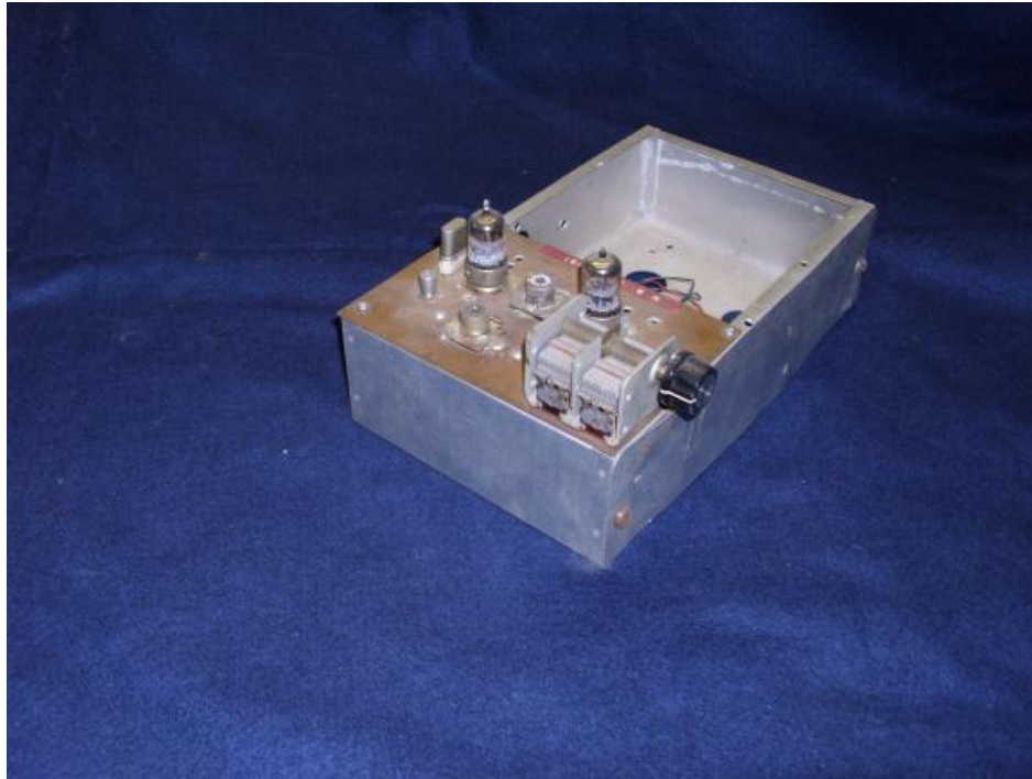
This converter changes the 160-meter band (1.8 to 2.0 MHz) to the 6-meter band (51.8 to 52.0 MHz)
