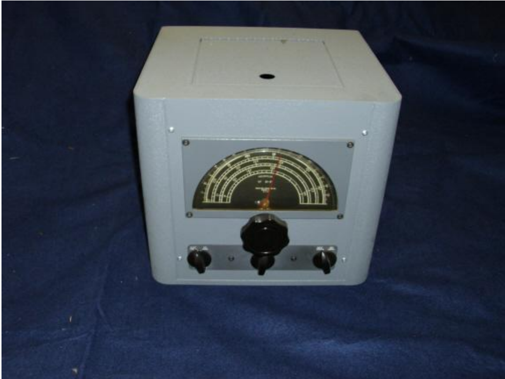
RME HF-10-20 (converts 20, 15, and 10 meter bands to 7.000 MHz)
