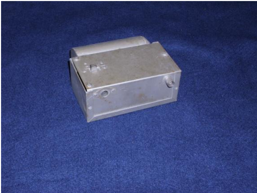
Home brew solid-state 6-meter mobile converter (early 1960s)
