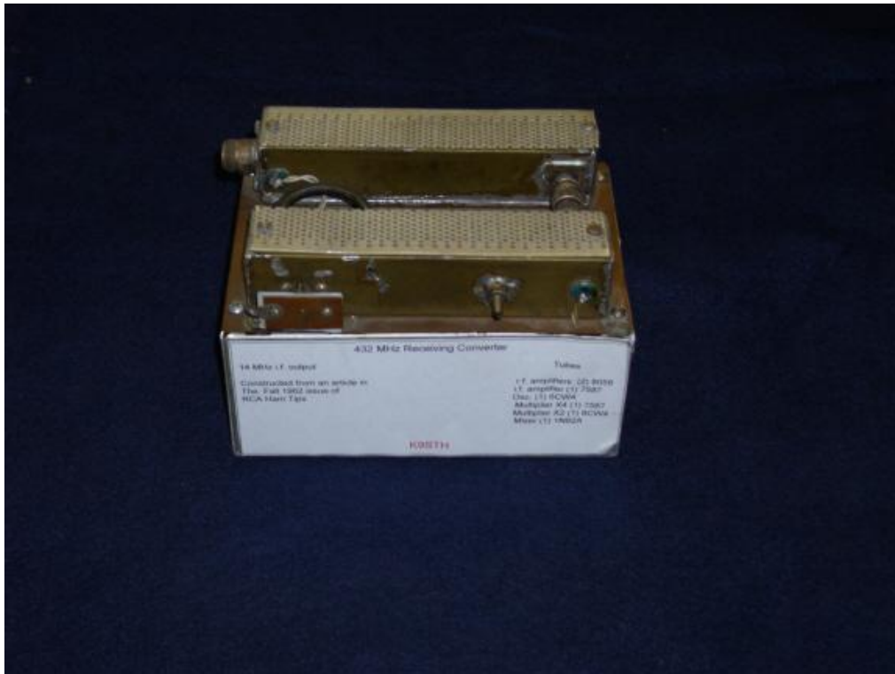
Home brew 432 MHz Nuvistor converter from RCA "Ham Tips" 1962
