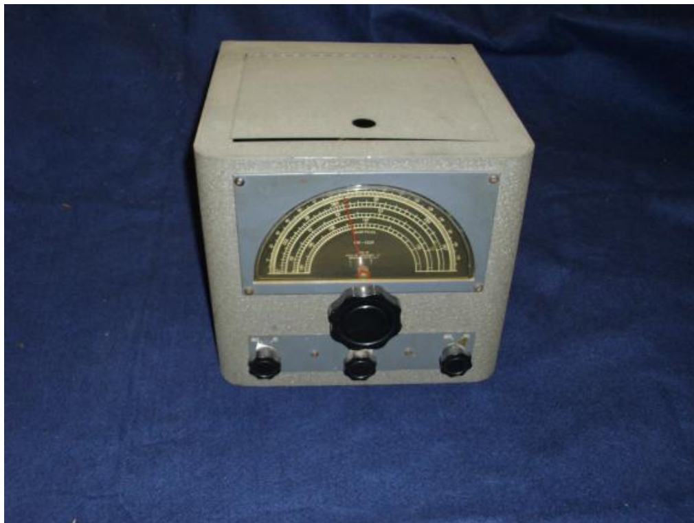
RME VHF-152 (converts 10, 6, and 2 meter bands to 7.000 MHz)
