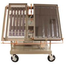
MODEL H-SST-4 Back view showing solar collector tilted toward sun
