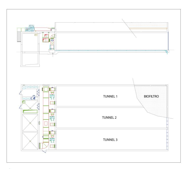
The plant uses the biotunnel composting technology for the biological treatment of organic waste deriving from the screening of mixed municipal waste.
