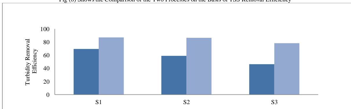
Fig (9) Shows the Comparison of the Two Processes on the Basis of Turbidity Removal Efficiency
