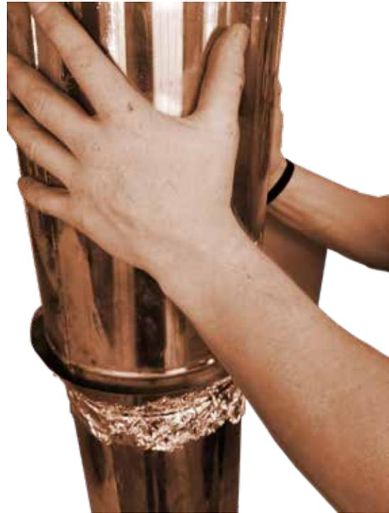
Flux along the seam of Cone and Pot and solder, go slow, in 3" stretches.
