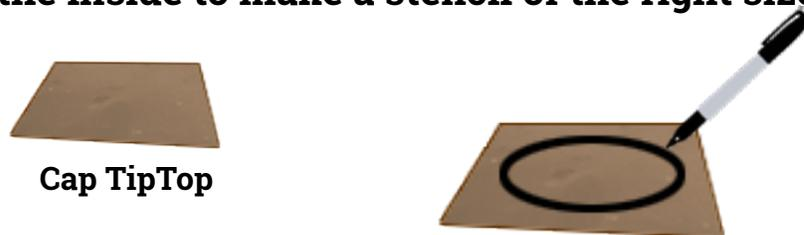
Cut the circle shape, leaving about a 1/8" extra when you cut, this will help make sure the circle you cut is not too small for the cap. Fit the circle into the top of Cap Kit, use something inside to drive the circle up and keep it in place while you solder (any metal cylinder would work).
