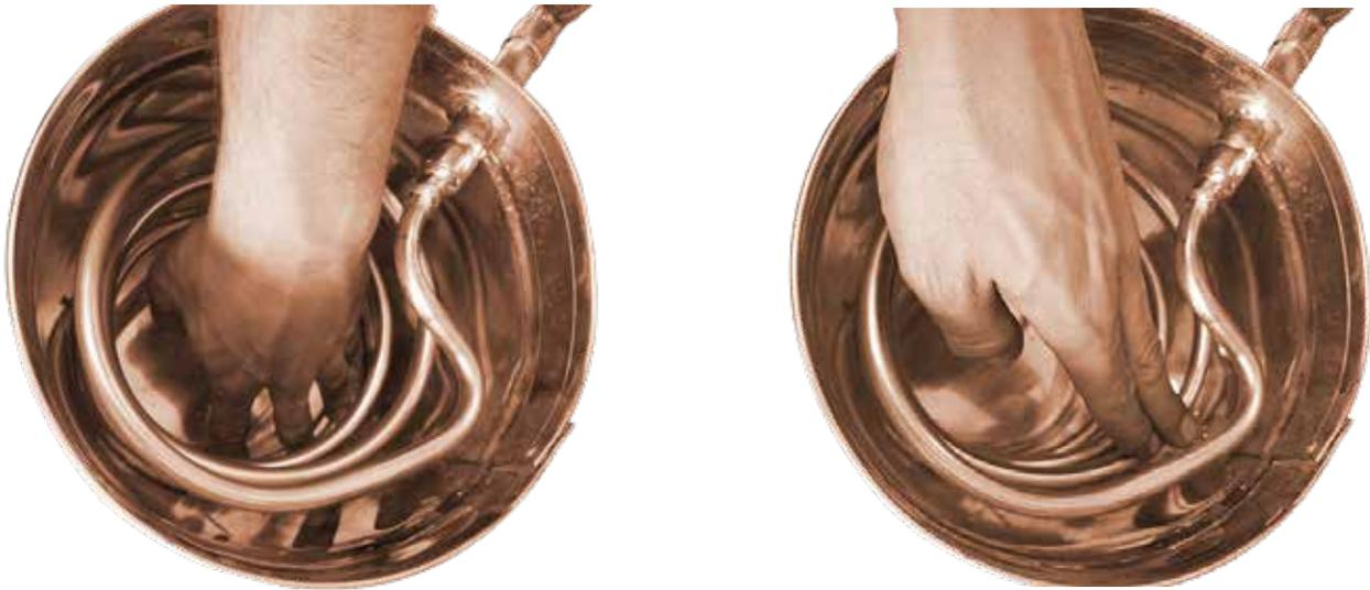
**Make sure when installing the coil, the flow of the spiral goes downwards to ensure the correct flow needed.**
