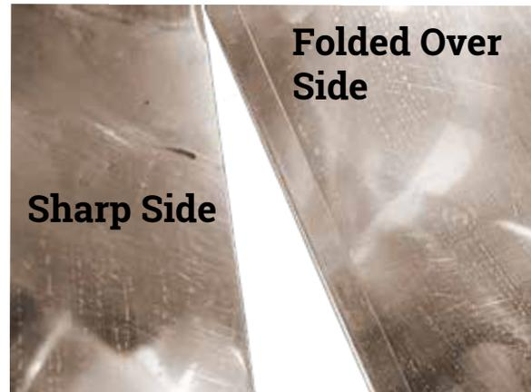
Flux the sharp side of the seam on the side facing towards you, flux the seam of the folded over side as well, just as we did with the pot.
