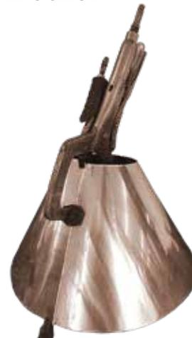
Flux and solder from the inside, make sure to fill the gaps well with the solder. Solder in two runs: the first run is to fill the gaps well; the second run is to make it look nice and even.
