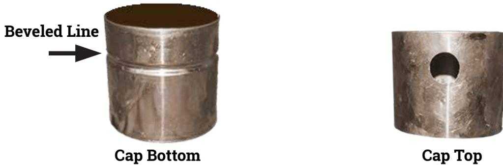
Flux the seams of Cap Top and Bottom; Insert the Cap top on Bottom with beveled line on top, match the seams as these interlock. Get the tightest fit you can, flux seams again and start soldering as you did with the pot.
