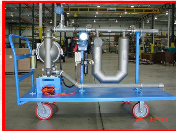
Aqueous Ammonia recirculation system with Micromotion flowmeter.
