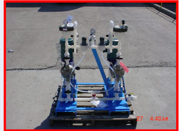
Chemical injection system utilizing Durameter metering pumps.
