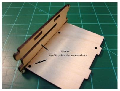
**One** – Line up side with base, use slot and holes to assist
