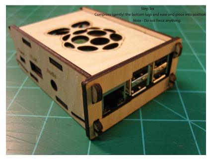
Six – Compress the bottom lugs gently and ease end plate into position. Be careful parts are delicate
