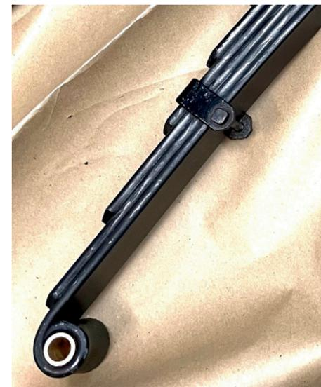
Front spring completed with dry lube paint, ready for finish
