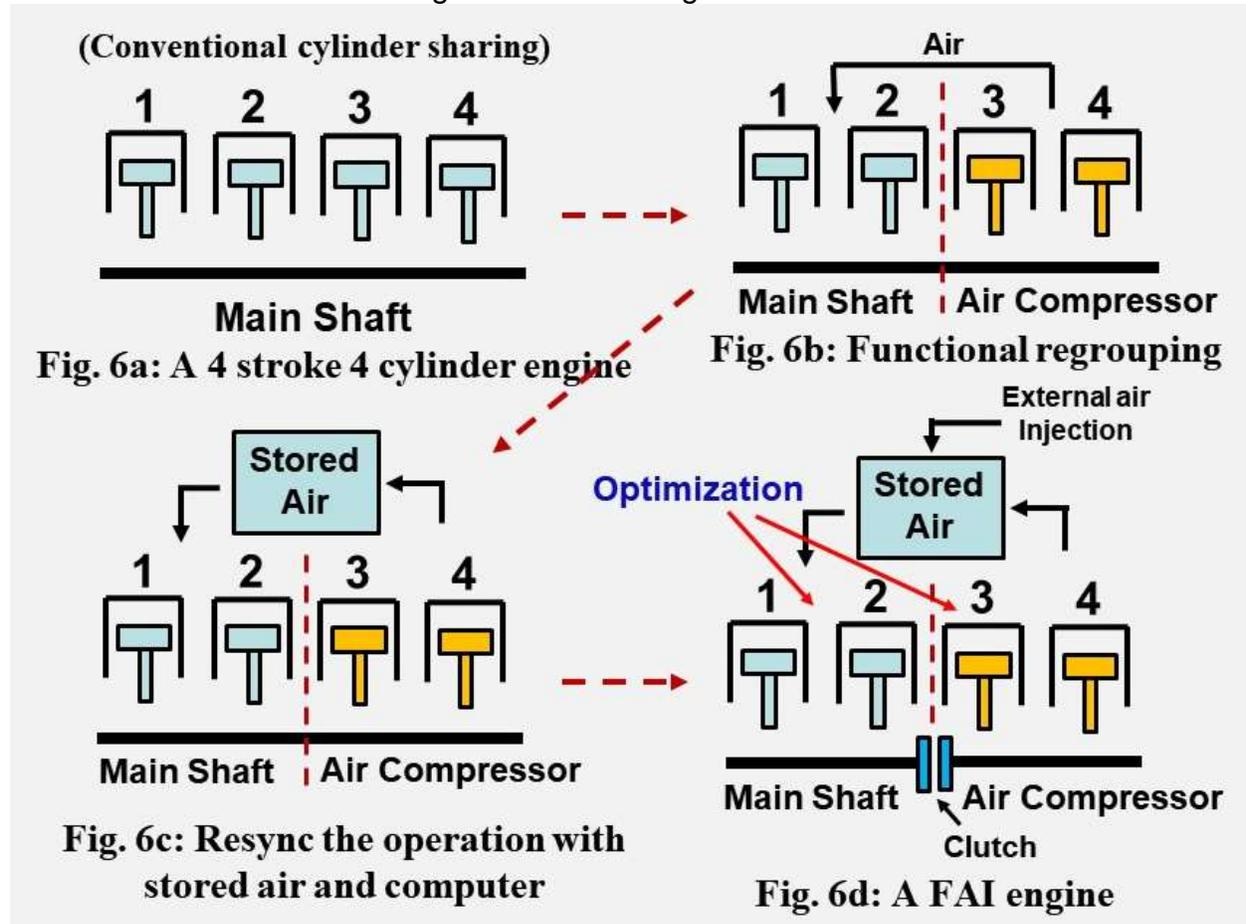
Fig. 6a represents a conventional 4-stroke 4-cylinder engine.
