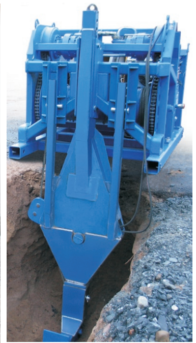
The 30 ton winch unit delivers enough power for even the heaviest pulling jobs.
