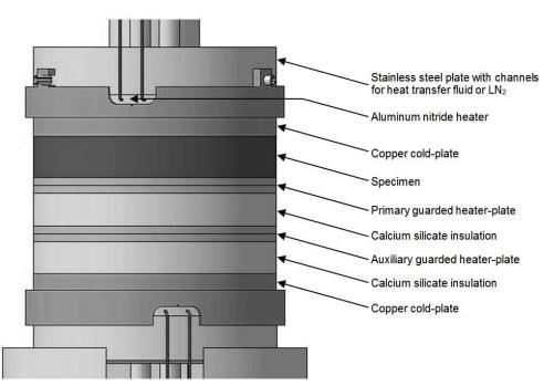
Temperature: - 100 ...  $250^{\circ}$  C Specimen: Ø 50.8 – 75 mm, 1 – 20 mm thick
