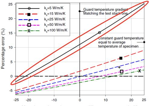
Meter bar and guard temperature difference on two ends (K)
