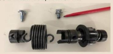
The other bolt is "special" only because it is only 11/16" long. This allows the bolt to lock the spring in place, without having the bolt actually touch the starter shaft. Don't be tempted to use a 3/4" long bolt instead of the correct shorter one. See the comparison photo of a 3/4" bolt and the correct bolt.
