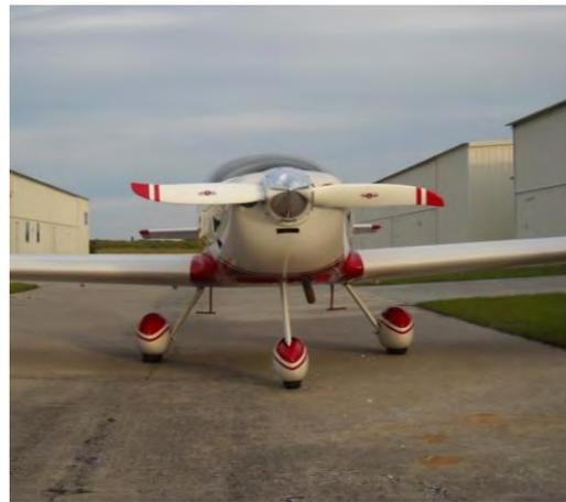
After a few hours at home, I changed out the landing and taxi lights for the Aeroleds 1600 in an effort to lower my amp usage. These light are bright and draw very little amps. I also added a trickle charger to the battery area so I could automatically charge the battery without having to remove any of the cowls. This has worked out to be good option for me.
