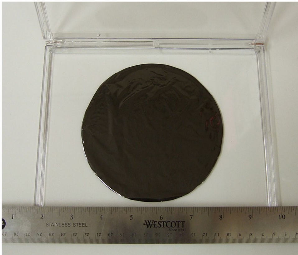
Photograph of a 13 cm diam. graphene film
