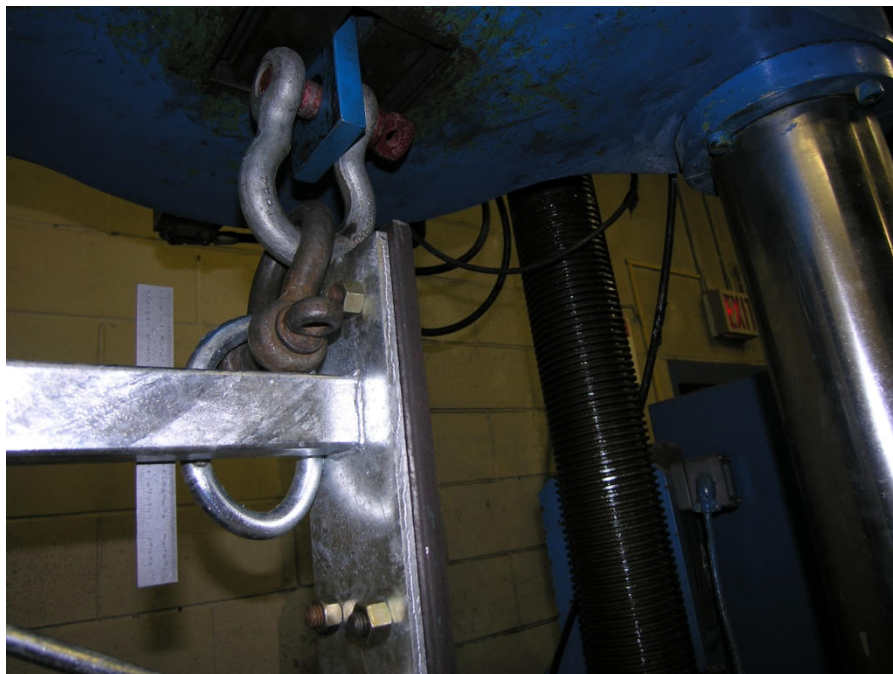
(b) Safety Loop Connection to Test Apparatus
