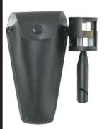
This compact and precise right angle prism allows for easy determination of right angle points or perpendicular points between two targets. The protective metal cover rotates to expose the pentagonal prisms.
