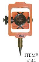
This 25 mm copper-coated prism features aluminum double yoke construction w/tilting coaxial target. There are on-board 130-minute vials, top & bottom. It includes replaceable plumb bob point. Height to center of prism w/plumb bob point: 100 mm.
