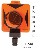
This is an all-metal, non-tilting prism holder with a 62-mm, sealed prism canister. The holder features both 0 and -30 mm offsets. The target/holder is constructed of durable aluminum and coated with corrosion-proof electrostatic paint, in fluorescent-orange.
