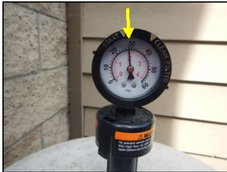
FYI - water pressure on the filter pump was 28 psi
