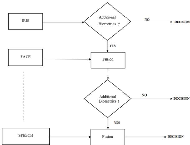
Fig.2: Serial Architecture
