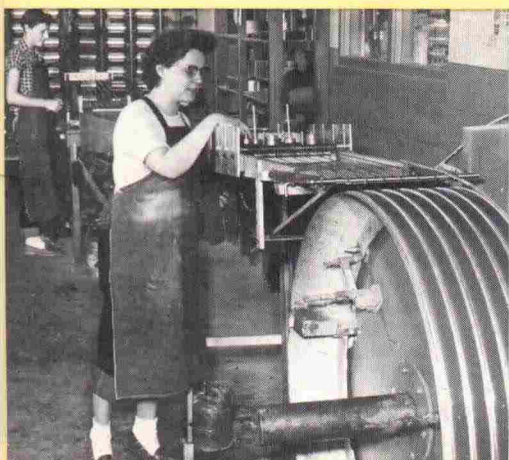
1. Bear "glass-power" in the making. Thousands of tough Fiberglas strands are bonded together, running full length of every bow.
