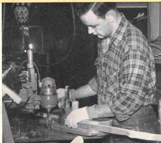
8. All the way through, human skill and precision machine work toward perfection. This high-speed router shapes recurve bow tips.
