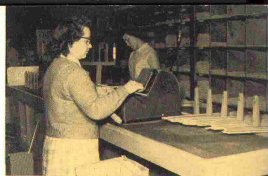
Selecting, weighing and classifying arrow shafts with aid of shadowgraph scale.
